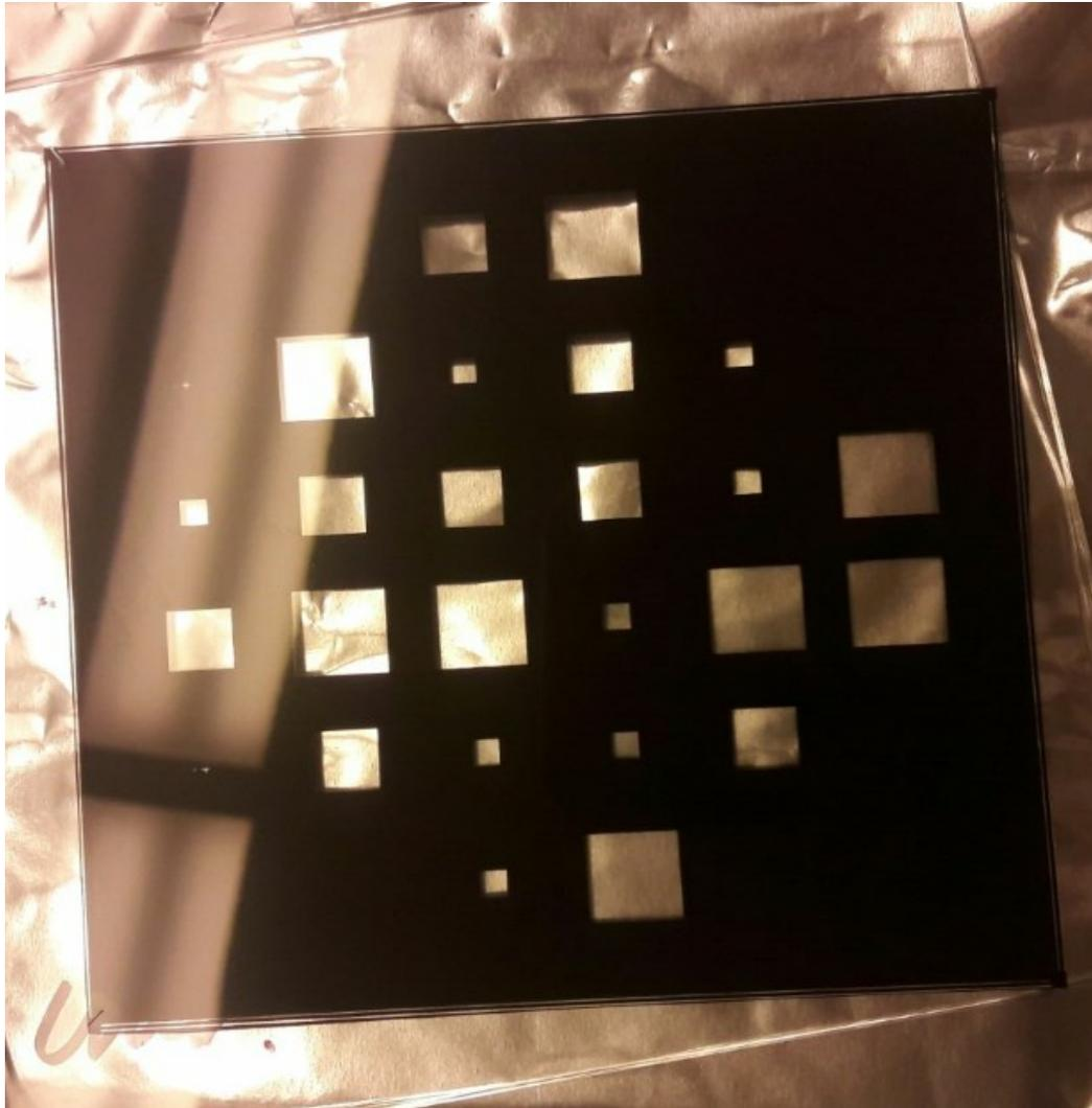
In our project, to ensure that there is no photoresist left on the windows, the second mask was exposed first, and following spray development, the second mask was exposed with a larger UV dose.
