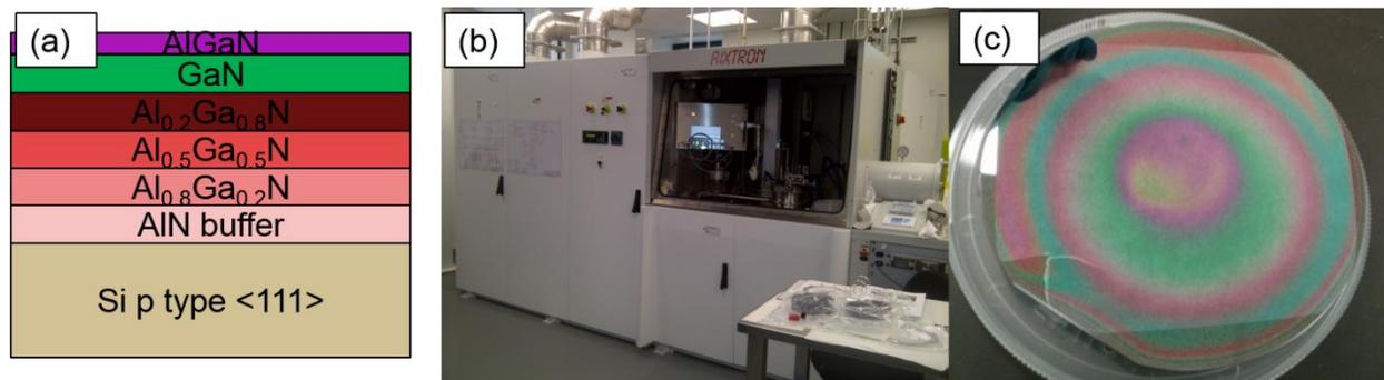
Figure 12 (a) Cross section of HEMT wafer films when grown on Si. (b) Image of the AAxitron metalorganic chemical vapor deposition system (MOCVD) (c) Image of the grown HEMT wafer.
