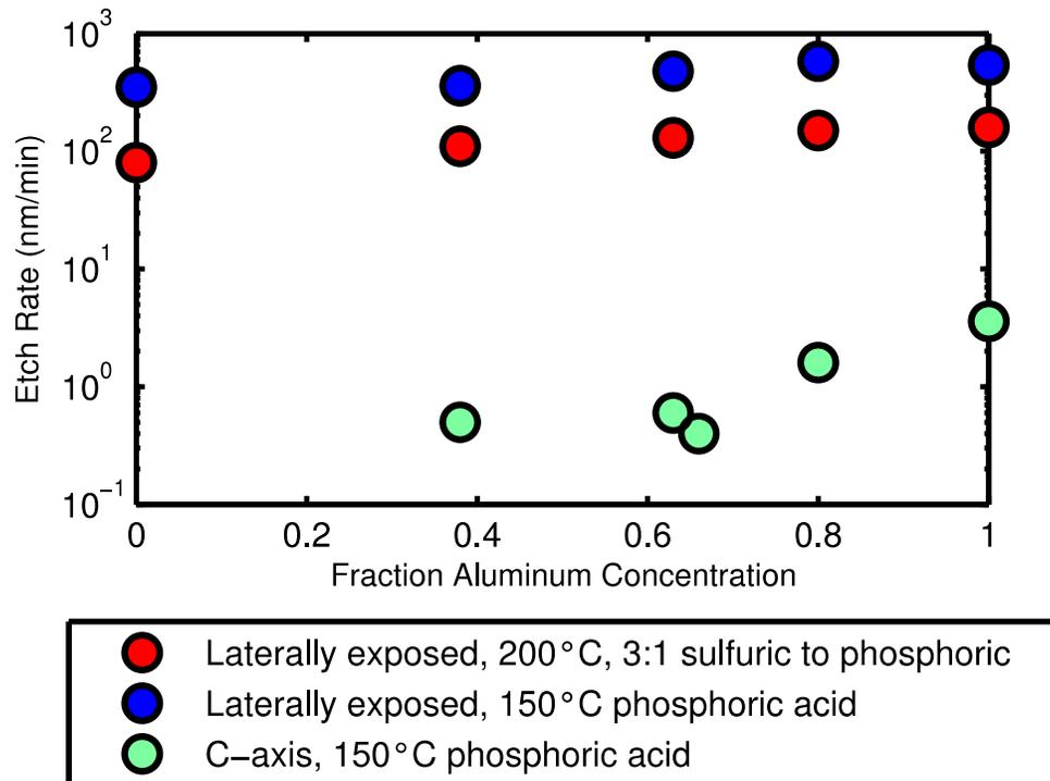
Figure 11 Summary of the vertical and lateral etch rates of GaN, AlGa<sub>n</sub>, and AlN with respect to aluminum concentration for phosphoric acid and sulfuric/phosphoric acid.
