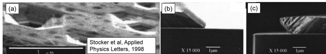
Figure 2 Previous work demonstrating anisotropic etching of MOCVD GaN. (a) GaN etched by 10% KOH in ethylene glycol. (b) GaN etched by  $\text{H}_3\text{PO}_4$  in the  $10\bar{1}3$  direction (c)  $\text{H}_3\text{PO}_4$  in the  $10\bar{1}2$  direction.
