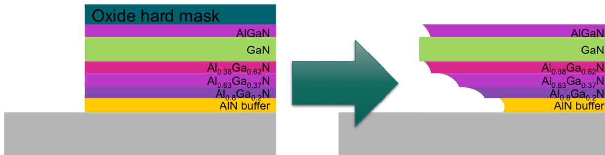
Figure 6 Schematic illustration of measurement method used to characterize lateral etch. The AlGaN/GaN HEMT layer was plasma etched in Ox III-V and then wet etched in a wet phosphoric etchant, revealing the anisotropic etch rate of the III-nitride films. The AlN buffer was hypothesized to etch faster in plane than the (Al)GaN layers.
