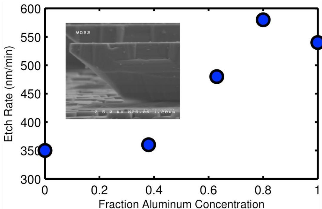
Figure 8 Lateral etch rates (parallel to 0001 crystal plane) in 150°C phosphoric acid for the AlGaIn/GaN HEMT layers varied with Al%. Inset is an SEM image of sample used for measurements.
