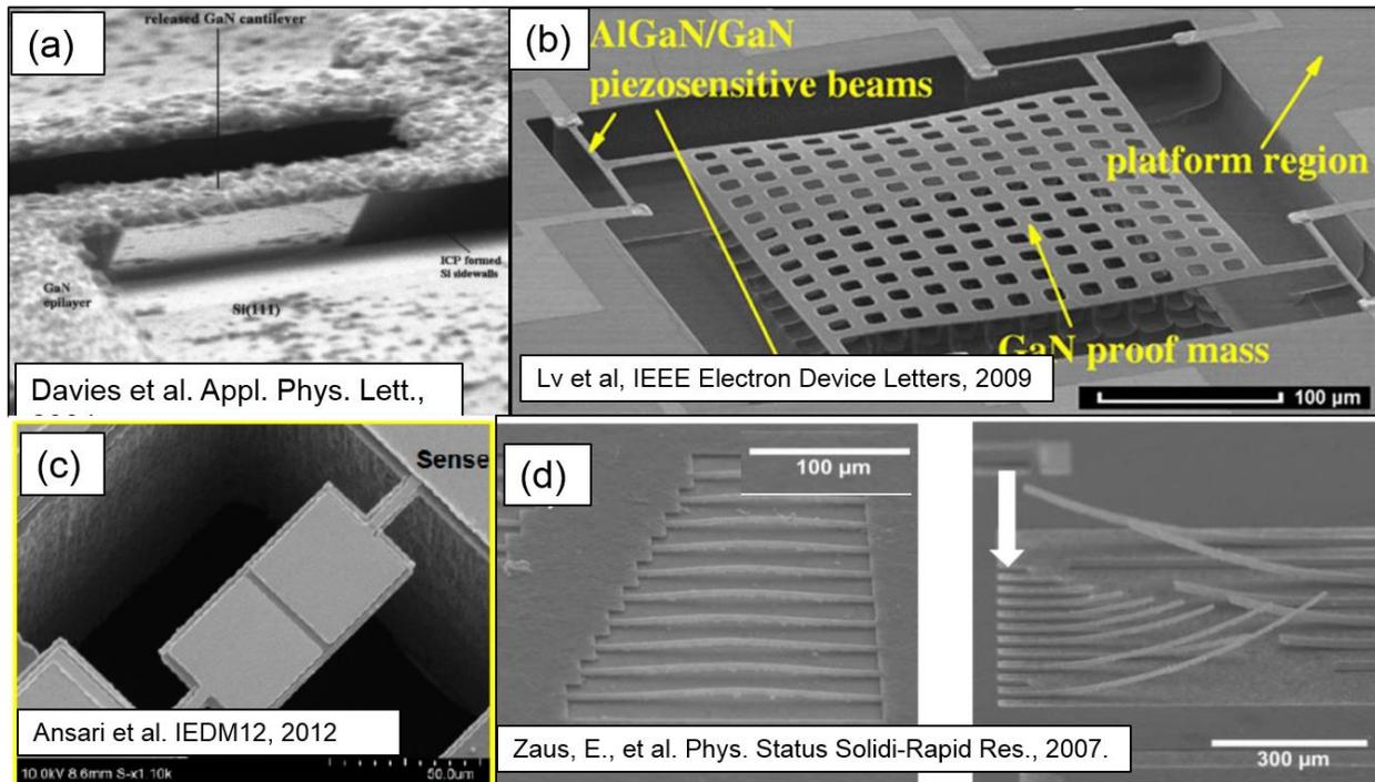
Figure 1 Previous work in the release of GaN and AlGaIn/GaN films. (a) MBE GaN/AlN on Si released by Si dry etch and KOH undercut. (b) MOCVD AlGaIn/GaN/AlN on Si released by SF<sub>6</sub> + O<sub>2</sub> plasma undercut. (c) MOCVD GaN/AlN on Si released by backside Si ICP etch. (d) MBE GaN/AlN on sapphire released by H<sub>3</sub>PO<sub>4</sub> wet etch
