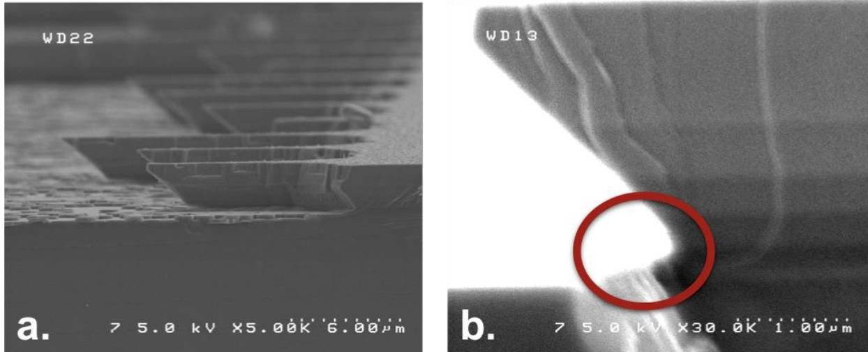
Figure 10 (a) SEM image of a pre-released cantilever array etched in 150 °C phosphoric acid for 5 minutes. (b) SEM image of a HEMT structure with undercutting also etched in 150 °C phosphoric acid for 45 minutes, revealing an AlN crystal plane with different dominant etch plane (~21°).
