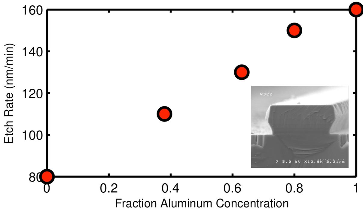
Figure 9 Lateral etch rates (parallel to 0001 crystal plane) in 200°C 3:1 sulfuric/phosphoric acid for the AlGaIn/GaN HEMT layers varied with Al%. Inset is an SEM image of sample used for measurements.
