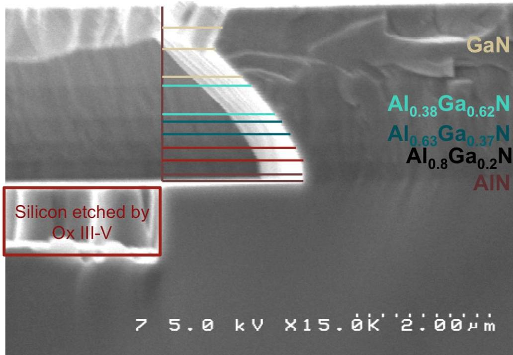
Figure 7 Cross section of the AlGaIn/GaN HEMT structure used for lateral etching characterization. This cross section is from the sample that was etch in 3:1 sulfuric/phosphoric acid. The dips into the silicon substrate on the bottom left are artifacts from the plasma etch step, and can be used as a reference line to measure lateral etch rates of each film.
