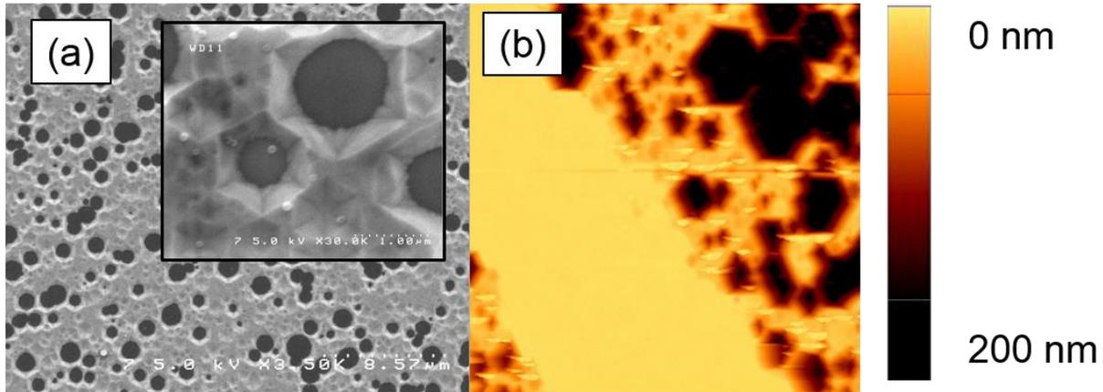
Figure 4 SEM of AlN sample etched for 5 minutes in 150 °C in phosphoric acid with inset of higher magnification, revealing hexagonal etch pits. (b) AFM image of the same AlN sample.
