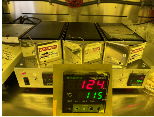
Figure 13: SNSF triple hotplate. Due to suboptimal feedback control, the temperature setting (green) can vary significantly from the temperature reading (red).
