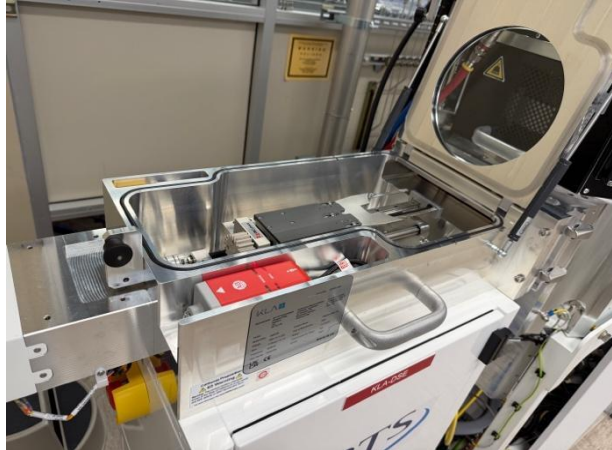
Fig. 9 — Lid lifted and held open, load lock arm exposed
