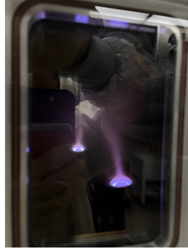
(b) Plasma in the chamber and Nb and Ti targets, Lesker2
