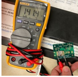
FIG. 15: Substrate with microheaters attached and wirebonded to carrier PCB.
