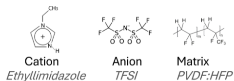
Figure 8. Chemical Structure of Ion Gel Electrolyte. EIM:TFSI (98% grade) was purchased from Iolitec and the PVDF-HFP pellets with an average weight-average molecular weight of ~400,000 were purchased from Sigma-Aldrich.
